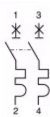
Internal schematic Diagram for Breaker
